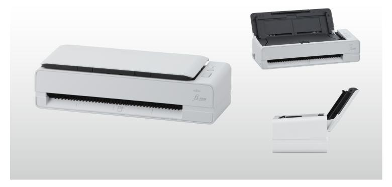
The fi-800R scans A4 portrait documents at comfortable speeds of 40 ppm/80 ipm (200/300 dpi) and makes customer onboarding easy with its compact size and versatile scanning abilities.
